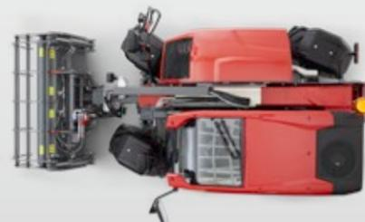
**Crab steering.** Sideways driving for ultra-precise maneuvering in confined spaces, such as when working against walls.
